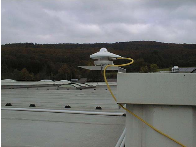
Fig. 3 shows the pyranometer used
